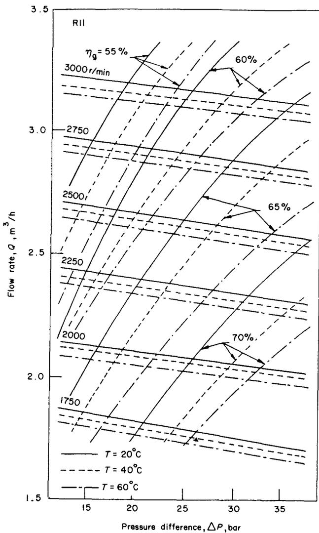
Fig 6 Pump map with R11 at 20, 40, 60 °C
