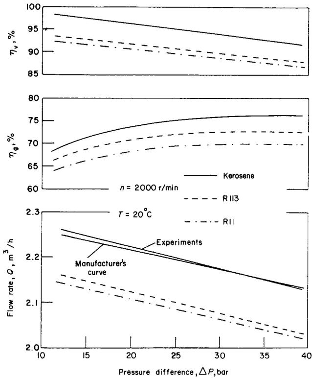
Fig 4 Head flow and efficiency curves at 2000 r/min for R11, R113 and kerosene at 20 °C
