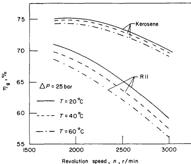
Fig 9 Pump overall efficiency as function of speed and fluid temperature
