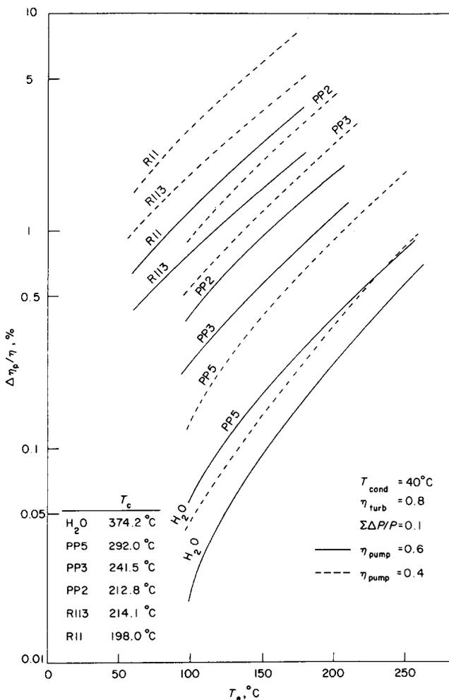
Fig 1 Pump efficiency incidence on cycle efficiency for different fluids
