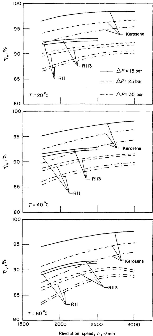
Fig 7 Pump volumetric efficiency at different speeds with R11, R113 and kerosene at various temperatures for different pressure difference
