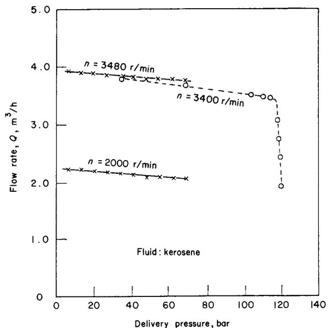
Fig 2 Pump calibration curve with kerosene.
