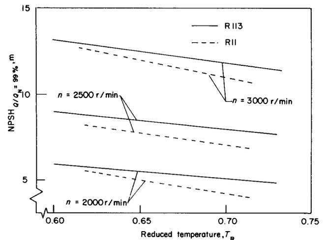
Fig 14 npsH values at  $Q/Q_N = 99\%$  against fluid reduced temperature
