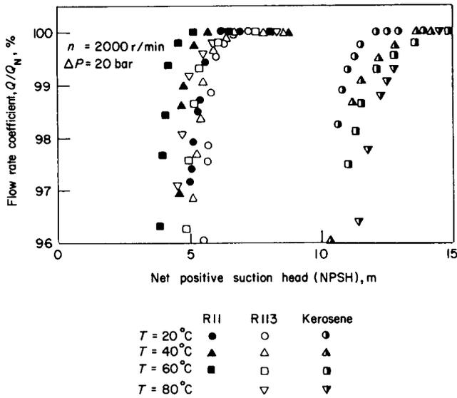
Fig 11 npsH values at 2000 r/min for R11, R113 and kerosene at various temperatures
