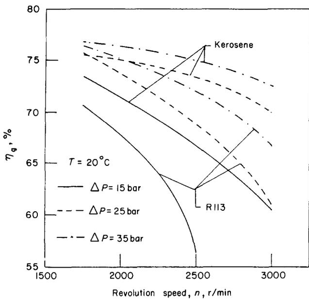
Fig 8 Pump overall efficiency as function of speed and delivery-suction pressure difference
