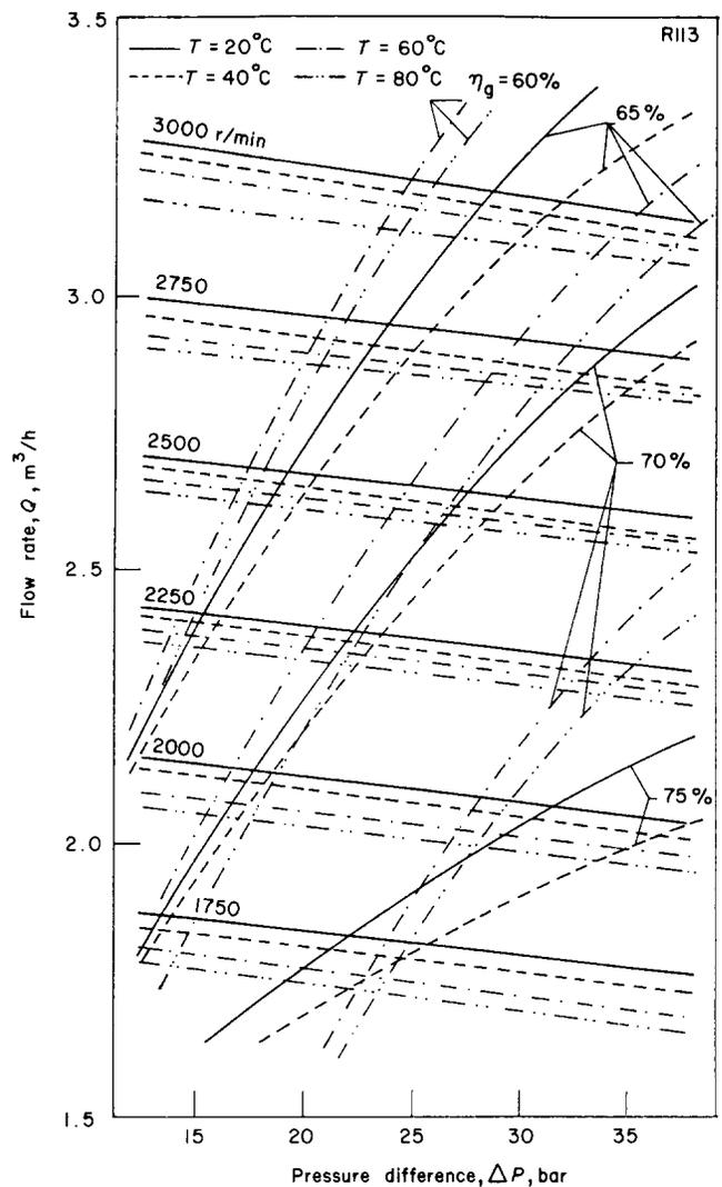
Fig 5 Pump map with R113 at 20, 40, 60, 80 °C
