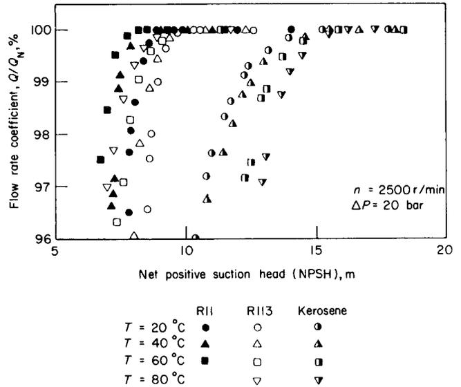
Fig 12 npsH values at 2500 r/min for R11, R113 and kerosene at various temperatures
