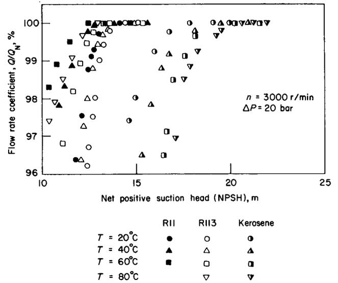
Fig 13 npsH values at 3000 r/min for R11, R113 and kerosene at various temperatures
