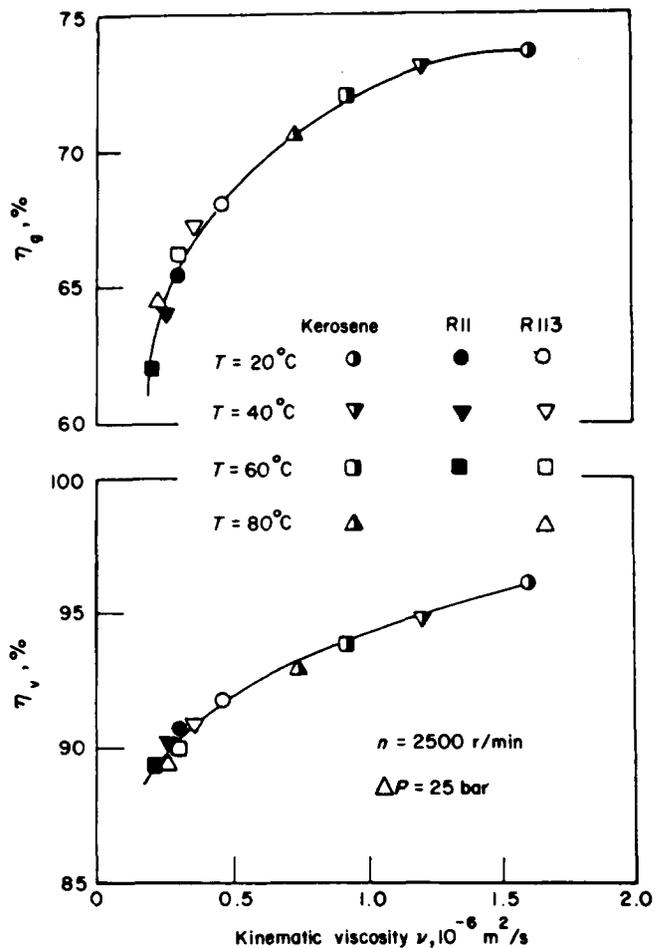
Fig. 10 Pump volumetric and overall efficiencies against kinematic viscosity
